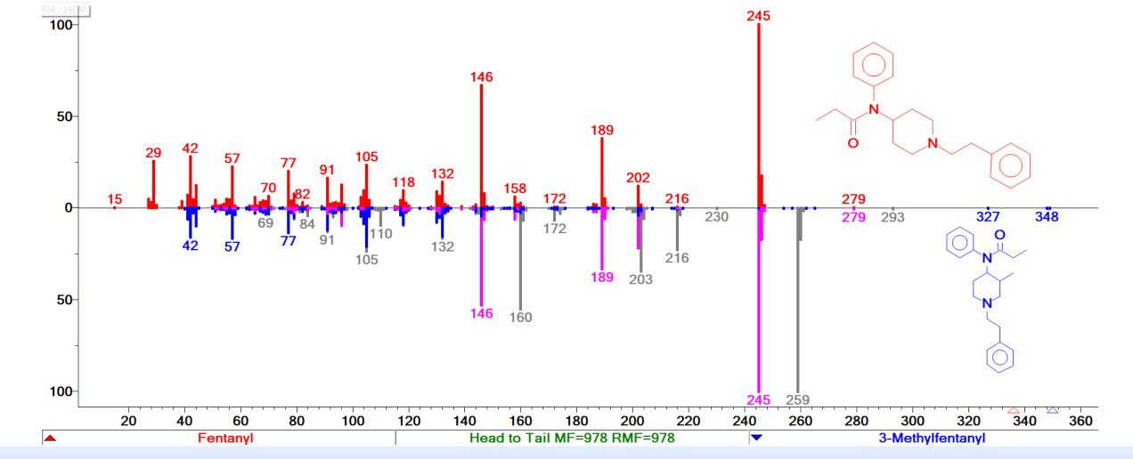
Shift peaks to match spectra for compounds that differ by an 'inert' chemical group. Both original and shifted peaks shown to aid structure analysis.
