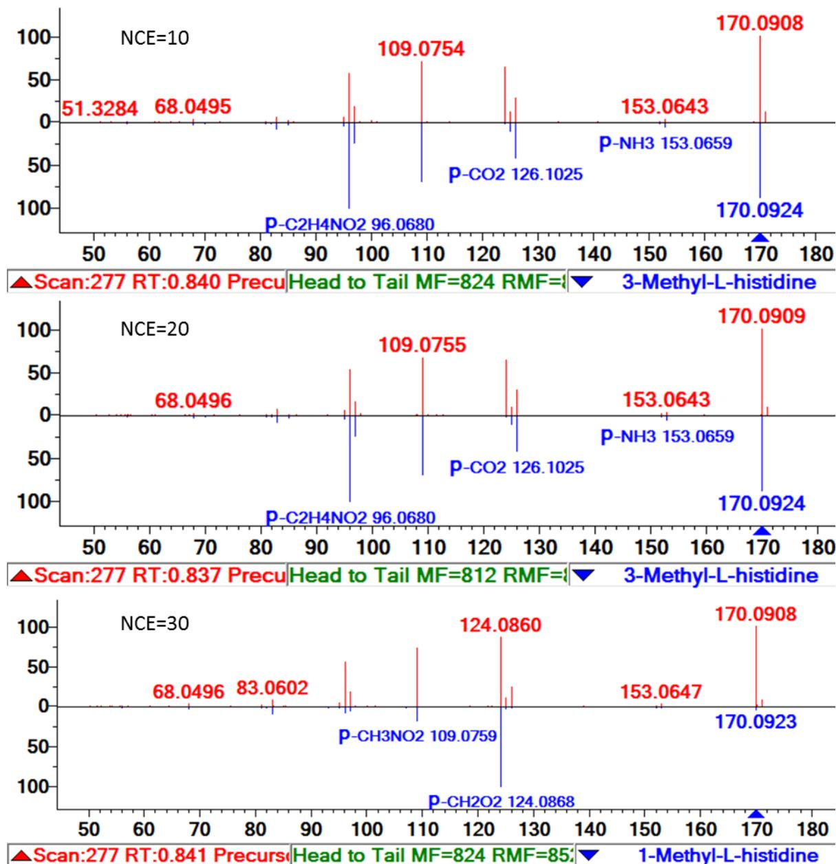
Figure 2. Spectra and library match of the same eluting mixture from experiments at different collision energies (10, 20 and 30 V). Note that best-matches are different at the lowest and the highest collision energy.
