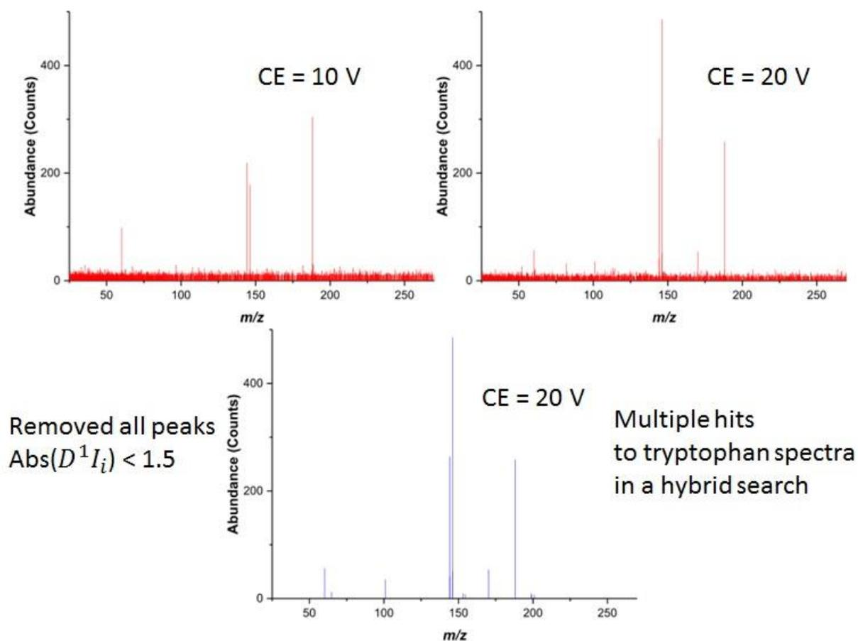
Figure 1. QToF MS<sup>2</sup>-spectra of N-acetyltryptophan at different collision energies (10 and 20 V). Denoised spectrum (below).
